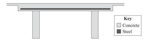
The tensile strength of concrete is very low compared with the tensile strength of steel.
