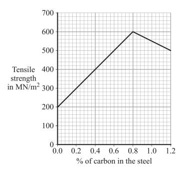
7A One type of steel has a tensile strength of  $400 \text{ MN/m}^2$ .
